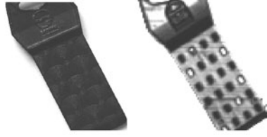
Figure 3. Picture (left) and THz peak-amplitude transmission image (right) of a plastic codekey.
