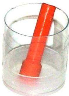
Figure 4.68. A vial and plastic tube were used for testing the T-ray CT system. An optical image of the target.
