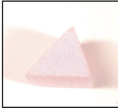
Figure 4.37. Simple polystyrene test target. The target consists of a triangular cylinder with a side length of approximately 1 cm.
