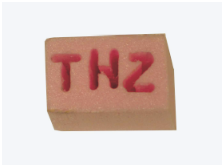
Figure 4.48. Polystyrene block with the letters 'THZ' drilled into it. This figure shows an optical image of the polystyrene block target. The target has dimensions of 45 \times 25 \times 35 mm (length \times width \times height) and the letters each have a thickness of approximately 2 mm.
