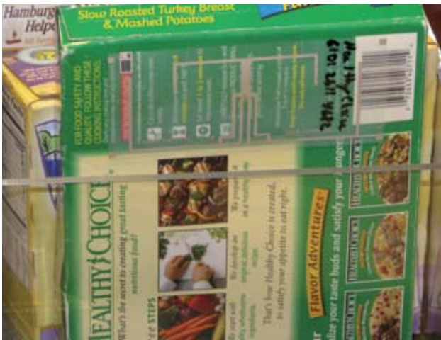
[ Location, location, location: optimum positioning of the tag on the item is a crucial determinant of RFID system performance. ]
