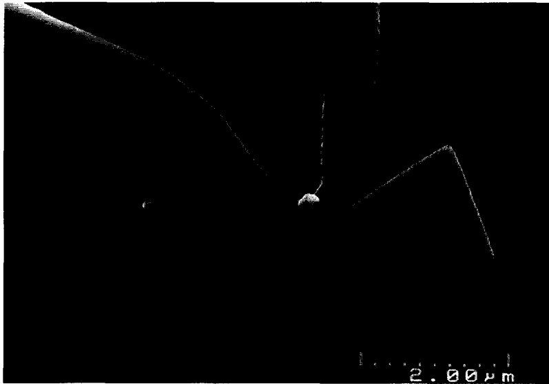
Fig. 1. Electron microscope image of our thin-film Ni–NiO–Ni diode with integrated bow-tie antenna taken at 45° incidence.
