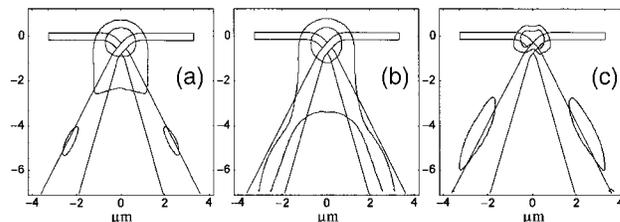
Fig. 3. Receiving area of the Ni-NiO-Ni diode for 633-nm radiation with polarization (a) parallel and (b) perpendicular to the antenna. (c) Difference between the parallel and the perpendicular polarizations. The contours correspond to 10% and 50% of the maximum value.
