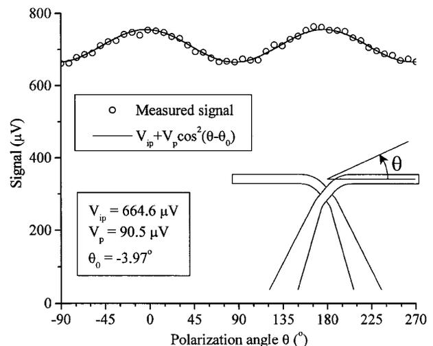
Fig. 1. Polarization dependence of the signal measured with an antenna-coupled Ni–NiO–Ni diode illuminated with 633-nm wavelength radiation.
