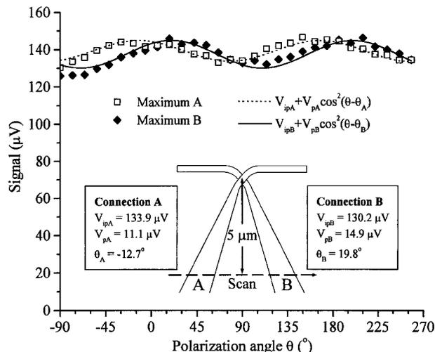
Fig. 2. Polarization dependence of the response of the connections to the diode.
