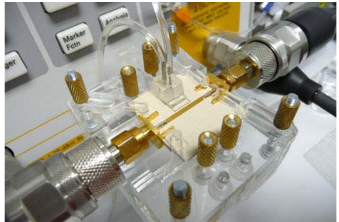
Figure 3. Photograph of the fabricated sensor in sample injection module.
