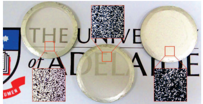
Fig. 1. A photograph of the fabricated beam-splitters. From left to right, beam-splitters with reflection to transmission ratios of 10:90, 50:50 & 90:10 in the terahertz range can be seen. The inserts show micrographs of the surface of the beam-splitters at a magnification of 60\times .
