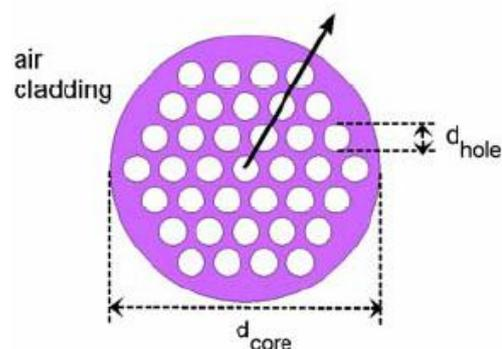
Fig. 1. Cross section and geometrical definitions of the triangular lattice porous fibre.
