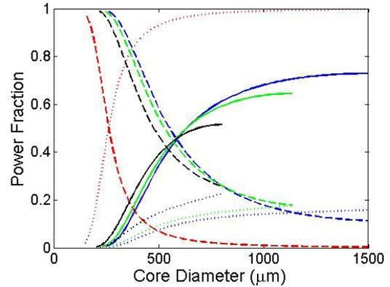
Fig. 3. Power fraction in the air holes (solid lines), core material (dotted lines) and air-clad (dashed lines) versus fibre diameter of a THz microwire (red lines) and porous fibres of 61% (black lines), 70% (green lines) and 74% (blue lines) porosity at  $f = 0.5 \text{ THz}$  ( $\lambda = 600 \mu\text{m}$ ).
