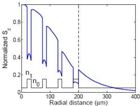
Fig. 2. The normalized Poynting vector,  $S_z$ , profile along the cross-section shown in Fig. 1., of the fundamental mode of a polymer porous fibre with core radius of  $d_{\text{core}}/2 = 200 \mu\text{m}$ , hole radii of  $d_{\text{core}}/2 = 20 \mu\text{m}$  and 37% porosity at  $f = 0.5 \text{ THz}$  ( $\lambda = 600 \mu\text{m}$ ). The dashed line represents the core to cladding interface and the lower solid line represents the refractive index profile.
