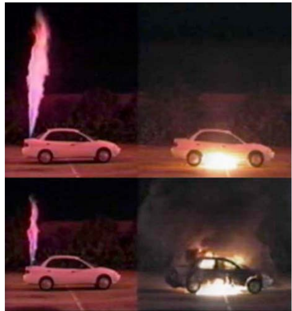
Fig. 6. On the left is a vehicle with a hydrogen tank, and on the right a vehicle with a standard gasoline tank. Both tanks have been deliberately punctured and ignited. The top panel shows the two vehicles 3 seconds after ignition. We see that, due to the buoyancy of hydrogen, the flame shoots up vertically, whereas gasoline is heavy and spreads beneath the vehicle. The bottom panel shows the two vehicles 60 seconds after ignition. The hydrogen supply has burned off and the flame is diminished, whereas the gasoline fire has accelerated and has totally engulfed the vehicle on the right. Note that hydrogen flames are not intrinsically visible, but salt and particles in the ambient air burn off giving color to the flame as seen above. Source: University of Miami.
