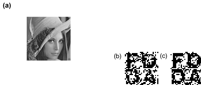
Figure 10. (a) The marked image 'Lena' after cropping as 300 \times 300 subpart. The recovered binary image S^* via (b) the isolated bistable detector, and (c) the array of bistable detectors with optimal noise intensity D_\eta/\Delta t = 200 . Here, \tau_a = T_b/150 , X_b = 3.75A and the array size N = 60 .
