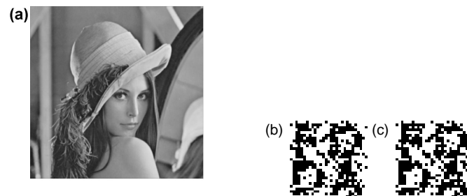
Figure 8. (a) The marked image 'Lena' filtered by a low pass filter with window size 2 \times 2 . The recovered binary image S^* via (b) the isolated bistable detector, and (c) the array of bistable detectors with optimal noise intensity D_\eta/\Delta t = 5 . Here, \tau_a = T_b/50 , X_b = 0.75A and the array size N = 60 .
