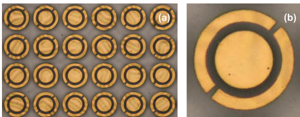
FIG. 2. Fabricated structure. Microscopic images for a small area (a) and a unit cell (b) of the converter with dimensions in agreement with Fig. 1(b).
