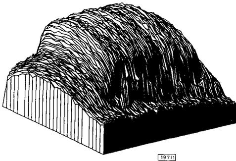
Fig. 1 MESFET drain current response to 2-D laser scan
