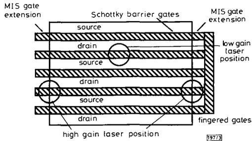
Fig. 3 Laser spot positions for high and low gain drain current response
