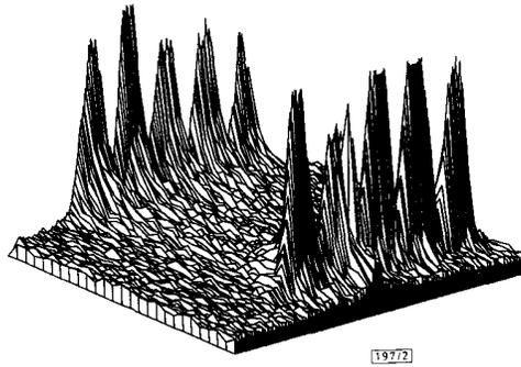
Fig. 2 MESFET drain current response to 2-D laser scan
