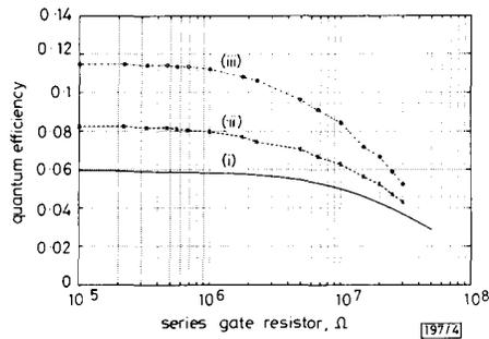
Fig. 4 Quantum efficiency against gate resistor
