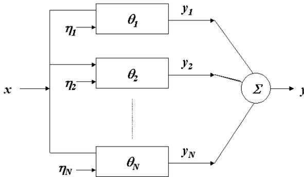
Fig. 1. Array of  $N$  summing comparators.
