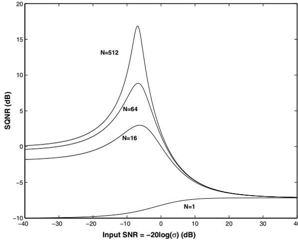
Fig. 4. Plot of SQNR in dB against the input SNR for various values of  $N$  and Gaussian signal and noise with  $c = 3\sigma_p$ .
