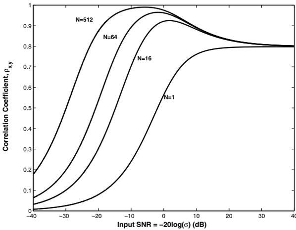
Fig. 3. Plot of Correlation Coefficient,  $\rho_{x,\hat{y}}$  against the input SNR for various values of  $N$  and Gaussian signal and noise.
