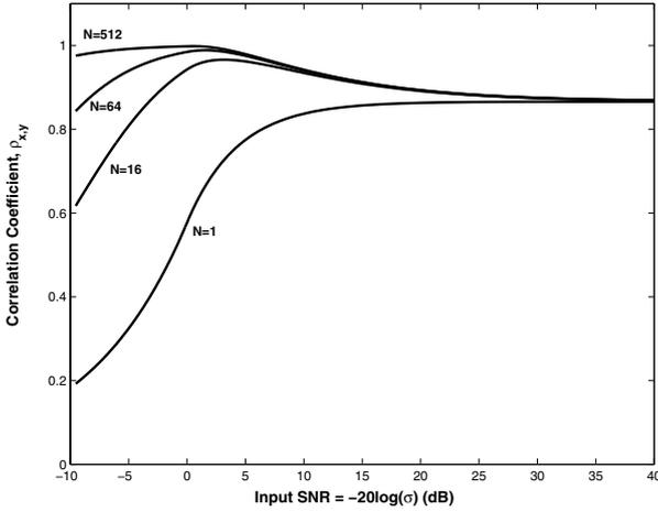
Fig. 2. Plot of Correlation Coefficient,  $\rho_{x,\hat{y}}$  against the input SNR for various values of  $N$  and uniform signal and noise.
