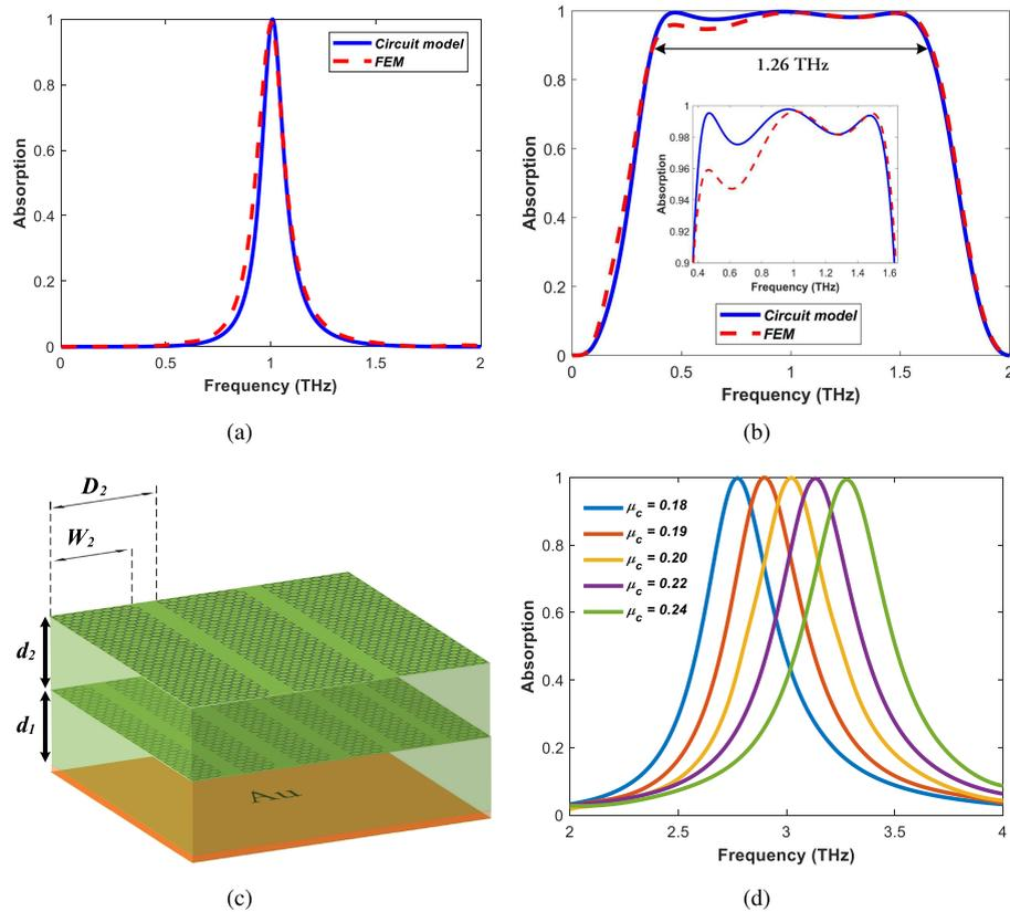
**FIGURE 6.** (a) Absorption spectra of the narrow band absorber with central frequency of  $f_0 = 1$  THz (Absorber 1 in Table 2) (b) ultra-wideband absorption spectra of the designed absorber with central frequency of  $f_0 = 1$  THz (the absorber in Table. 3), (c) configuration of ultra-wideband absorber with two PAGRs (The absorber in Table. 3), and (d) absorption spectra of absorber 2 in Table 2 with tunability of the peak's frequency, calculated by FEM.
