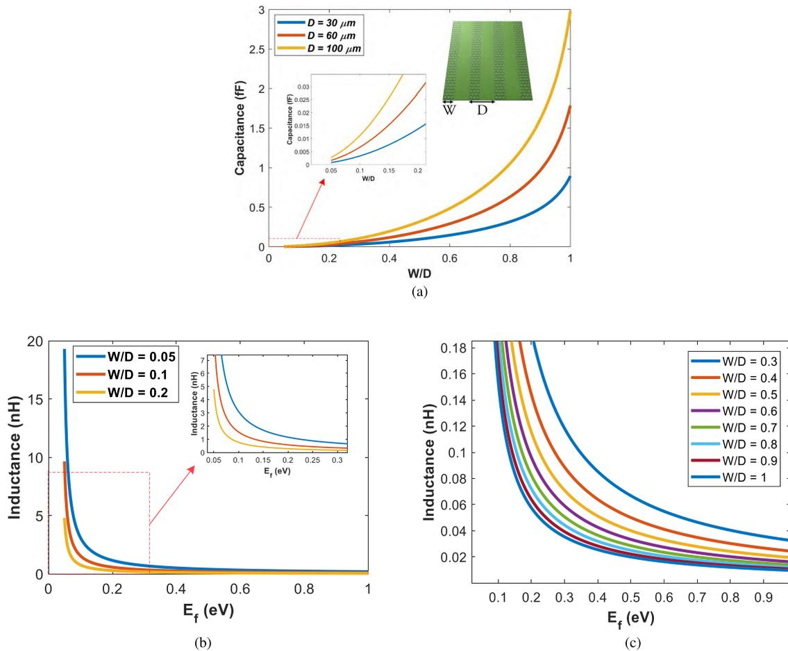
**FIGURE 3.** (a) Capacitance of the PAGRs ( $C_1$ ) as a function of  $W/D$  ratio (b) inductance of the PAGRs ( $L_1$ ) as a function of graphene Fermi energy with  $D = 100 \mu\text{m}$  (c) inductance of the PAGRs ( $L_1$ ) as a function of graphene Fermi energy with  $D = 100 \mu\text{m}$ .
