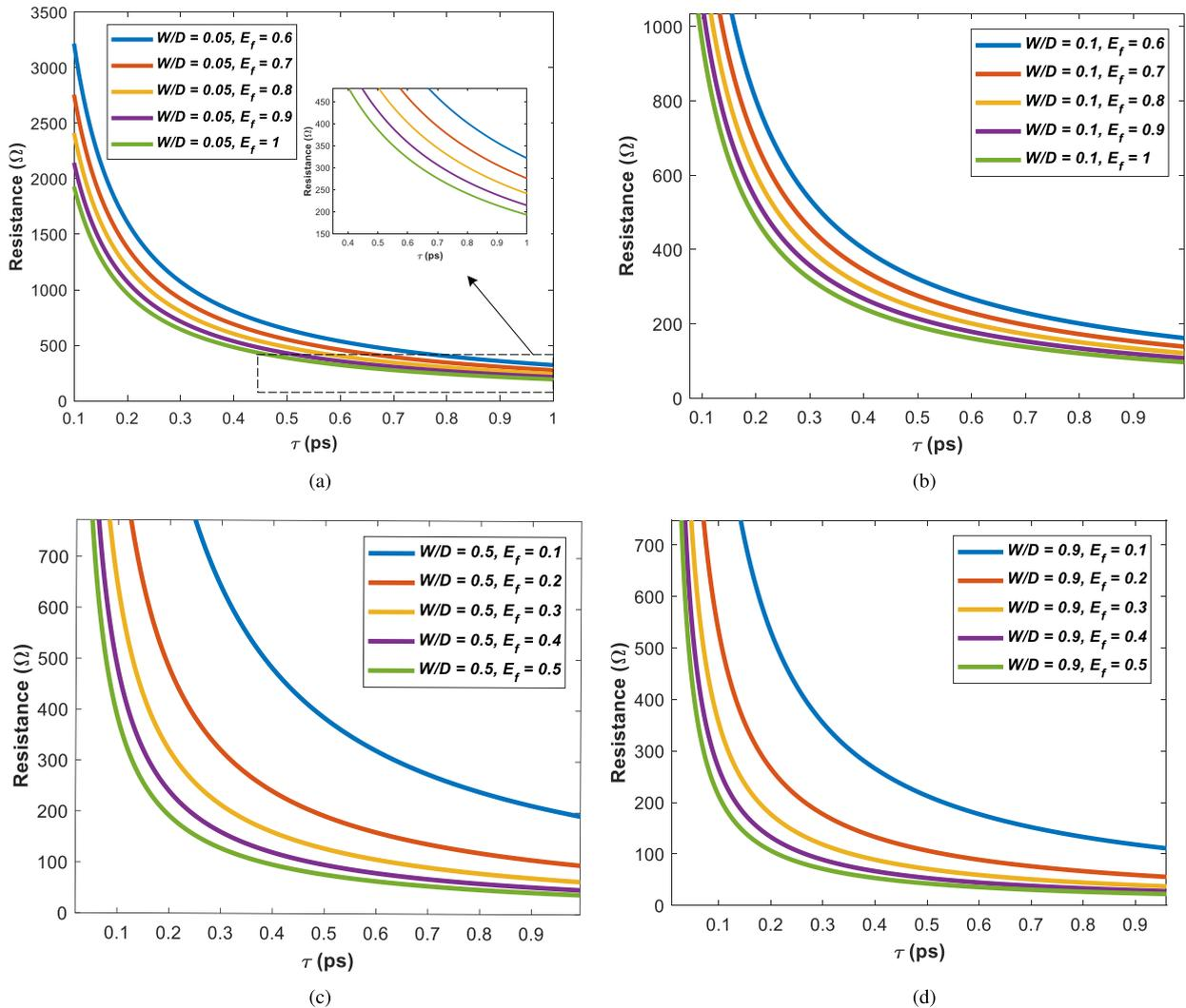
**FIGURE 4.** (a) Resistance of the PAGRs ( $R_1$ ) as a function of graphene relaxation time with  $D = 100 \mu\text{m}$  (b) Resistance of the PAGRs ( $R_1$ ) as a function of graphene relaxation time with  $D = 100 \mu\text{m}$  (c) Resistance of the PAGRs ( $R_1$ ) as a function of graphene relaxation time with  $D = 100 \mu\text{m}$  (d) Resistance of the PAGRs ( $R_1$ ) as a function of graphene relaxation time with  $D = 100 \mu\text{m}$ .
