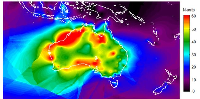
**FIGURE 5.** Ordinary kriging of  $dN_{75mH}$  from the 50 closest stations, with a power model  $\gamma(h) = b|h|^{0.7}$ , for the Australian region. Leakage of high overland values to the ocean to the south-west is seen, and discontinuity where high-value stations are included or excluded from the kriging system.
