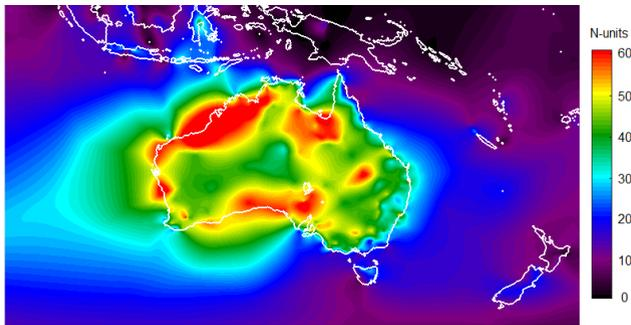
**FIGURE 6.** Natural neighbour interpolation, with added points to eliminate vertex circumcircle radius ratios exceeding 5:1, of parameter  $dN_{75mH}$ . While leave-one-out testing suggests these added points improve accuracy, the contours in ocean areas appear to be less smooth than the conventional technique, and leakage of land values into ocean areas may be increased.
