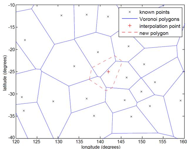
**FIGURE 2. Natural neighbour interpolation: an example showing the Voronoi polygons corresponding to the known points, overlapped by a new polygon for a location to be interpolated. The interpolation weights are proportional to the six areas of overlap of the original polygons.**
