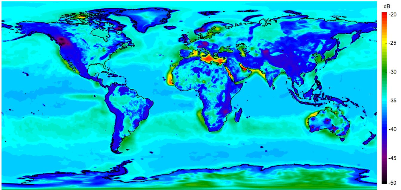
FIGURE 9. Worldwide map of geoclimatic factor  $K_G$ , produced by universal kriging. This indicates predicted severity of multipath fading.
