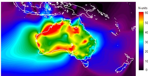
**FIGURE 7.** Conventional natural neighbour interpolation of weather station parameter  $dN_{75mH}$ . A smooth interpolated surface is obtained even though only a small number of local points are used in each interpolation.
