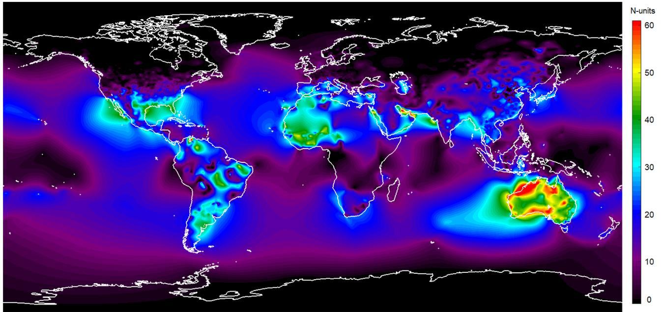
**FIGURE 8.** Worldwide map of the Harvey model for worst-case radio refractivity increase with height in the lowest 75 m of the atmosphere,  $dN_{75\text{mH}}$ .
