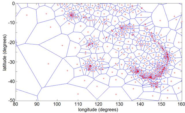
**FIGURE 4.** Voronoi polygons for surface weather stations in the Australian region, with additional interpolated “quasi-stations” to eliminate very irregular polygons. These interpolated points are added at polygon vertices until no polygon has vertex circumcircle radii spanning a ratio exceeding 5:1.
