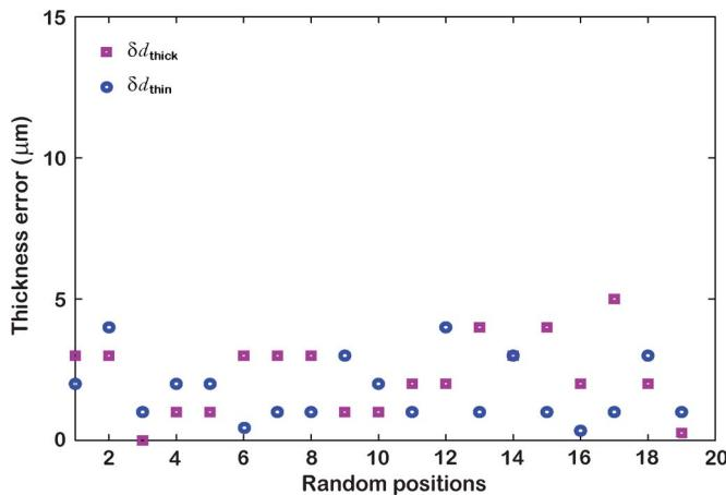
Fig. 10. Sample thickness error present at random positions in the thin and thick liquid layer of the fixed dual-thickness liquid sample holder. This plot shows that the  $\delta d$  for thin and thick liquid layer is less than  $5 \mu\text{m}$ .
