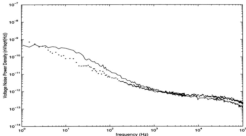
Fig. 2. Curves of PSD of device #131 with  $g-r$  noise (solid) and device #12 without  $g-r$  noise (dotted).
