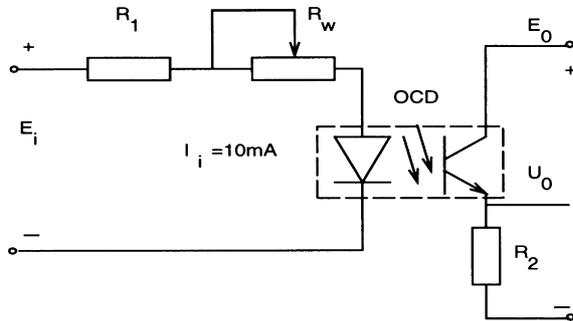
Fig. 1. Measuring circuit for optoelectronic coupled devices.
