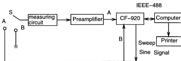
Fig. 3. The measurement system block diagram.
