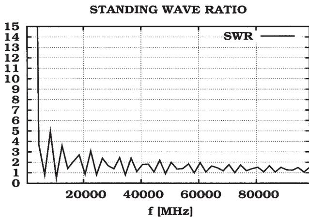
**Figure 8** SWR of the 5<sup>th</sup> antenna in Table 1 (less than five at 20–100-GHz bandwidth)
