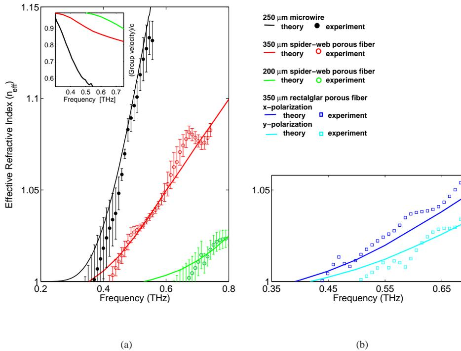
Fig. 6. Effective refractive index of a 200  $\mu\text{m}$  (green) and a 350  $\mu\text{m}$  (red) diameters of spider-web porous fiber, a 250  $\mu\text{m}$  diameter microwire (black) and a 350  $\mu\text{m}$  diameter of rectangular porous fiber  $x$ -polarization (blue) and  $y$ -polarization (cyan) as a function of frequency. The solid lines represent the theoretical results based on the real fiber while the circles represent the measured experimental results.
