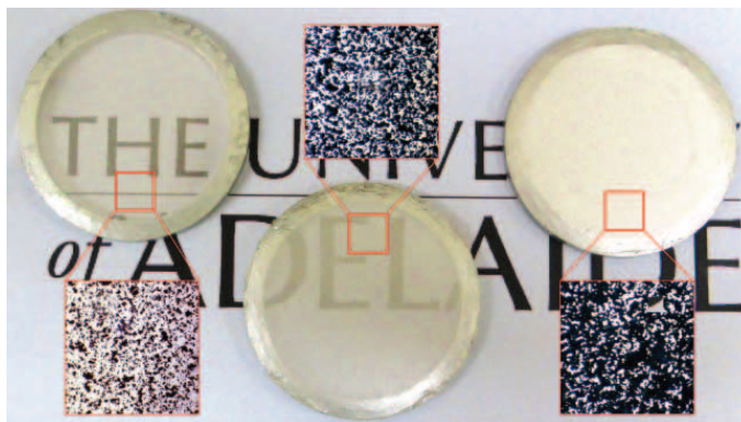
Fig. 3. Photograph of the fabricated beam-splitters. From the left, beam-splitters are shown with a terahertz reflection/transmission ratio of 10:90, 50:50 & 90:10. The expanded views show photos from a microscope camera showing the surface of the silver conductive paint layer at a magnification of 60\times . These microscope photos show that the area of the LDPE is covered more than 10% and 50% for the 10:90 and 50:50 ratio beam-splitters respectively, demonstrating that they are not area based polka-dot beam-splitters.
