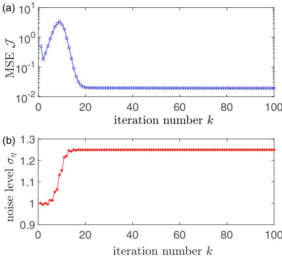
FIG. 6. Learning curves of (a) MSE  $\mathcal{J}$  of the 5-order filter of Eq. (17) and (b) the level  $\sigma_\eta$  of the added noise. Here, the initial level  $\sigma_\eta(0) = 1$  of the added noise and the other parameters are the same as in Fig. 4.
