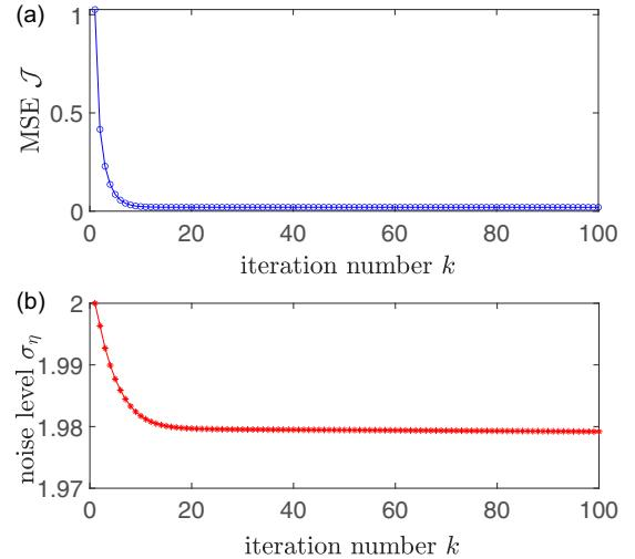
FIG. 4. Learning curves of (a) MSE  $\mathcal{J}$  of the 5-order filter of Eq. (17) and (b) the level  $\sigma_\eta$  of the added noise. The learning rate  $\mu = 5$  for updating the weight  $w$ , 0.01 for the noise level  $\sigma_\eta$ , and 0.001 for the threshold  $\gamma$ . Here, the initial noise level  $\sigma_\eta(0) = 2$ , the initial weight vector  $\mathbf{w}(0) = [1, -1, -1, -1, -1]^\top$ , and the initial threshold  $\gamma(0) = 0$ .
