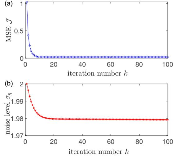
FIG. 4. Learning curves of (a) MSE  $\mathcal{J}$  of the 5-order filter of Eq. (17) and (b) the level  $\sigma_\eta$  of the added noise. The learning rate  $\mu = 5$  for updating the weight  $\mathbf{w}$ , 0.01 for the noise level  $\sigma_\eta$ , and 0.001 for the threshold  $\gamma$ . Here, the initial noise level  $\sigma_\eta(0) = 2$ , the initial weight vector  $\mathbf{w}(0) = [1, -1, -1, -1, -1]^\top$ , and the initial threshold  $\gamma(0) = 0$ .
