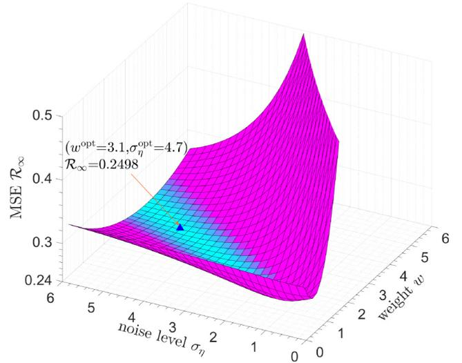
FIG. 2. MSE  $\mathcal{R}_{\infty}$  in Eq. (7) as a function of the weight  $w$  and the noise level  $\sigma_{\eta}$  for a given quantizer threshold  $\gamma = 0$ . The minimum  $\mathcal{R}_{\infty} = 0.2498$  ( $\blacktriangle$ ) at the optimal weight  $w^{\text{opt}} = 3.1$  and the optimal level  $\sigma_{\eta}^{\text{opt}} = 4.7$  of the added Gaussian noise is marked.
