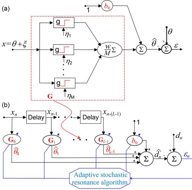
FIG. 1. Block diagram representations of (a) the summing threshold network model  $G$  for the noise-enhanced estimator  $\hat{\theta}$  and (b) the adaptive noise-enhanced transversal filter  $\hat{d}_n$ .
