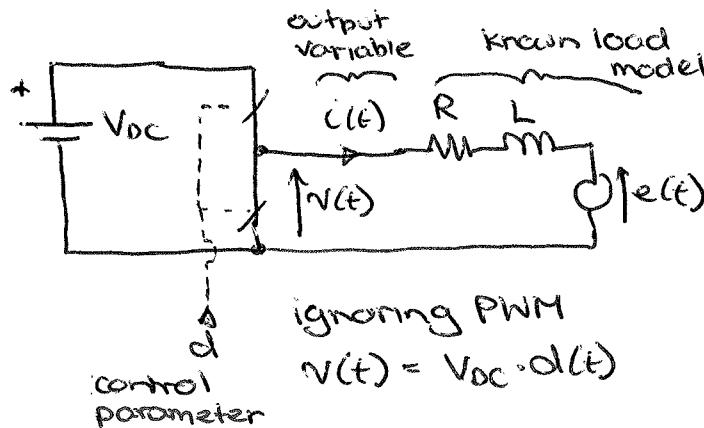
can use duty-cycle to command a desired output voltage  $V^*(t)$
