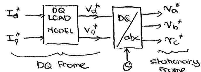
Feedforward offers good transient performance but prone to steady-state errors due to model errors
