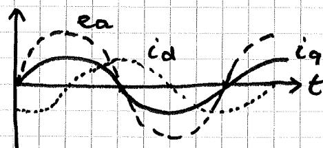
q-axis current  $i_q$  is in-phase with  $e$
