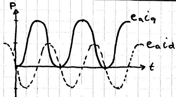
only the q-axis current produces average power in a surface PM machine
