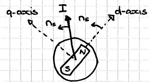
stator current phasor is not rotating relative to the rotor
