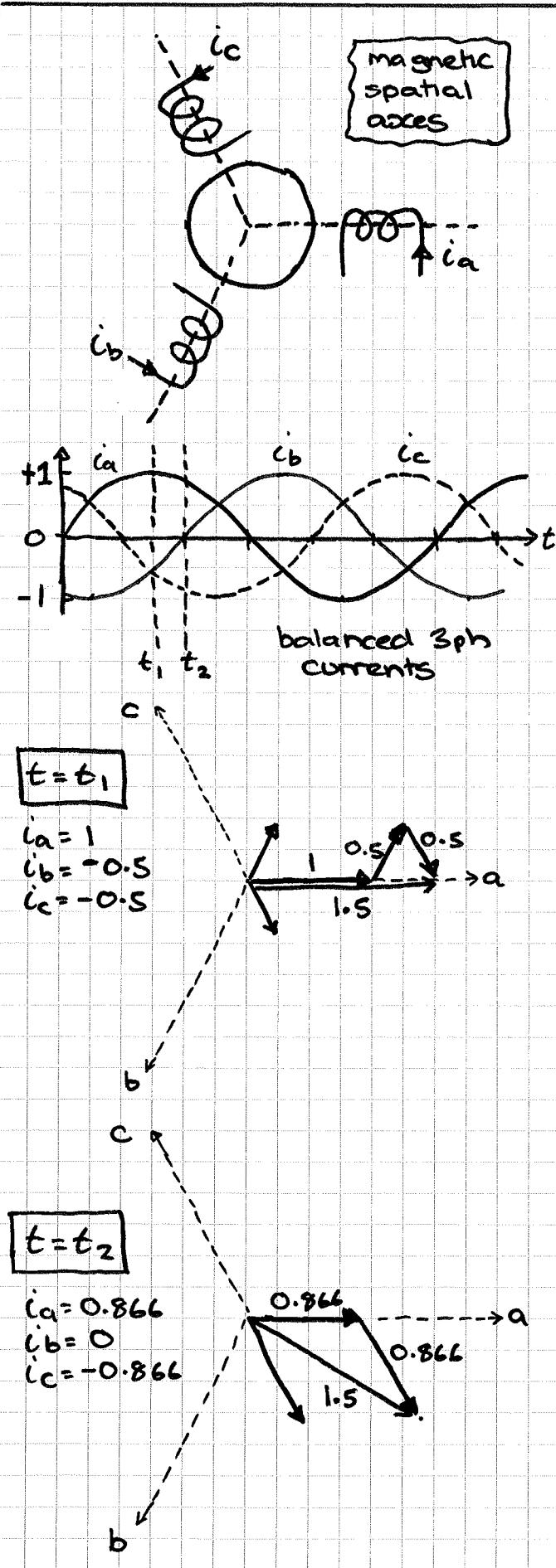
three phase balanced currents in three windings create a rotating magnetic field at synchronous speed whose magnitude is 1.5 times that produced by the peak field produced by each phase alone.
