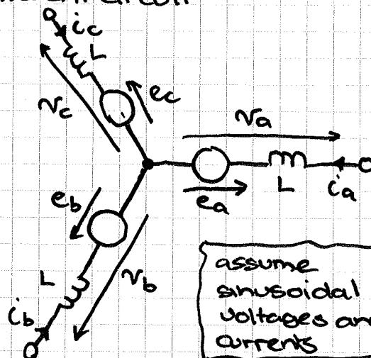
voltages and currents in each phase are balanced: equal magnitudes  $120^\circ$  out of phase
