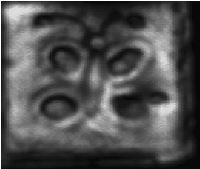
Fig. 5. Time-domain power integration of THz-beam reflection from plaster/graphite/plaster interface. The graphite image of a butterfly, extracted from between plaster layers, is clearly recognizable.
