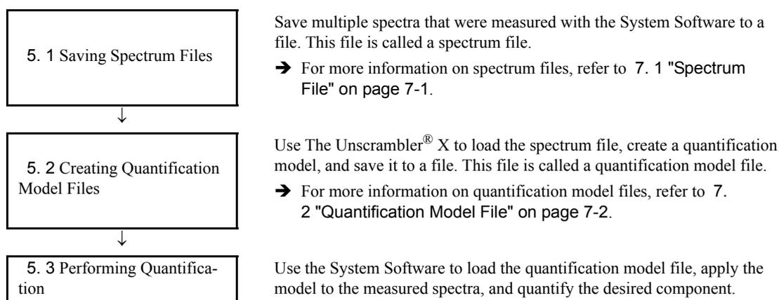
If the quantification model file already exists, the procedures described in 5. 1 "Saving Spectrum Files" on page 5-1 and 5. 2 "Creating Quantification Model Files" on page 5-4 are not needed.
