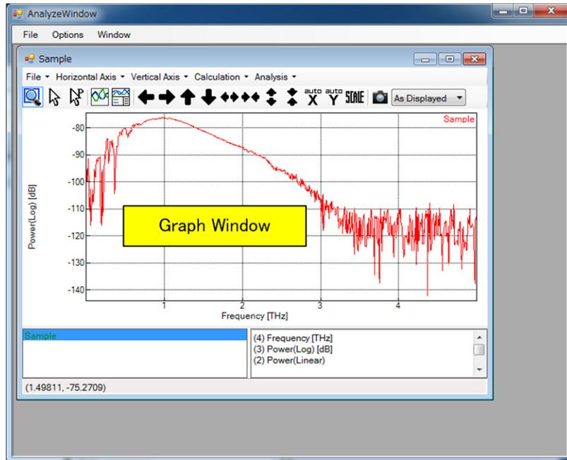
3) Change the type of vertical axis for the spectrum.
