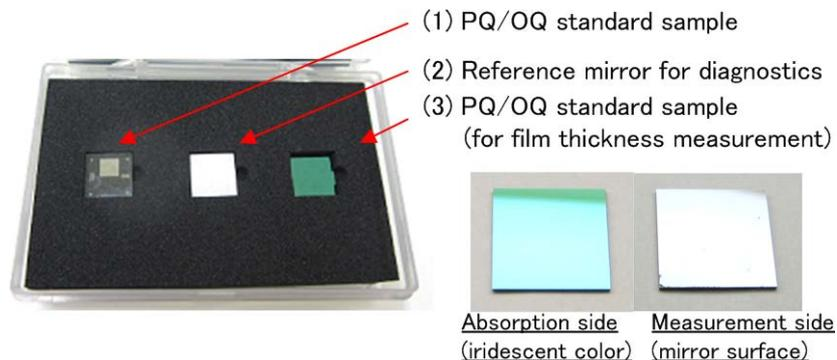
**Figure 6-4 How to Set Standard Sample**
