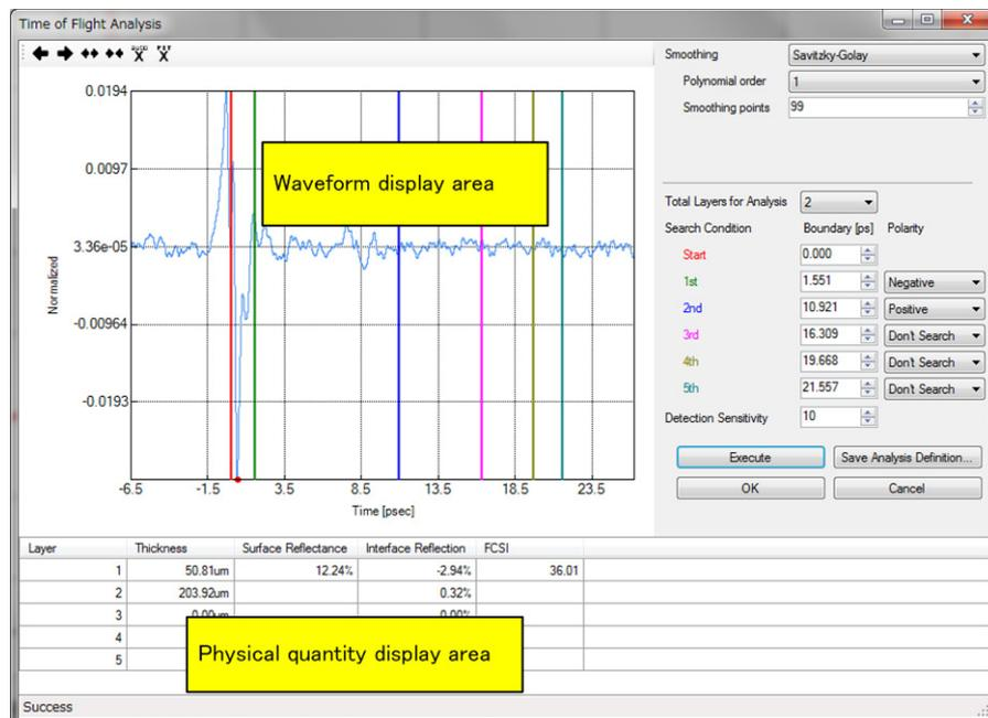
c) Select **[File]** → **[Save Analysis Definition...]** in the graph window to save the analysis parameters to file.
