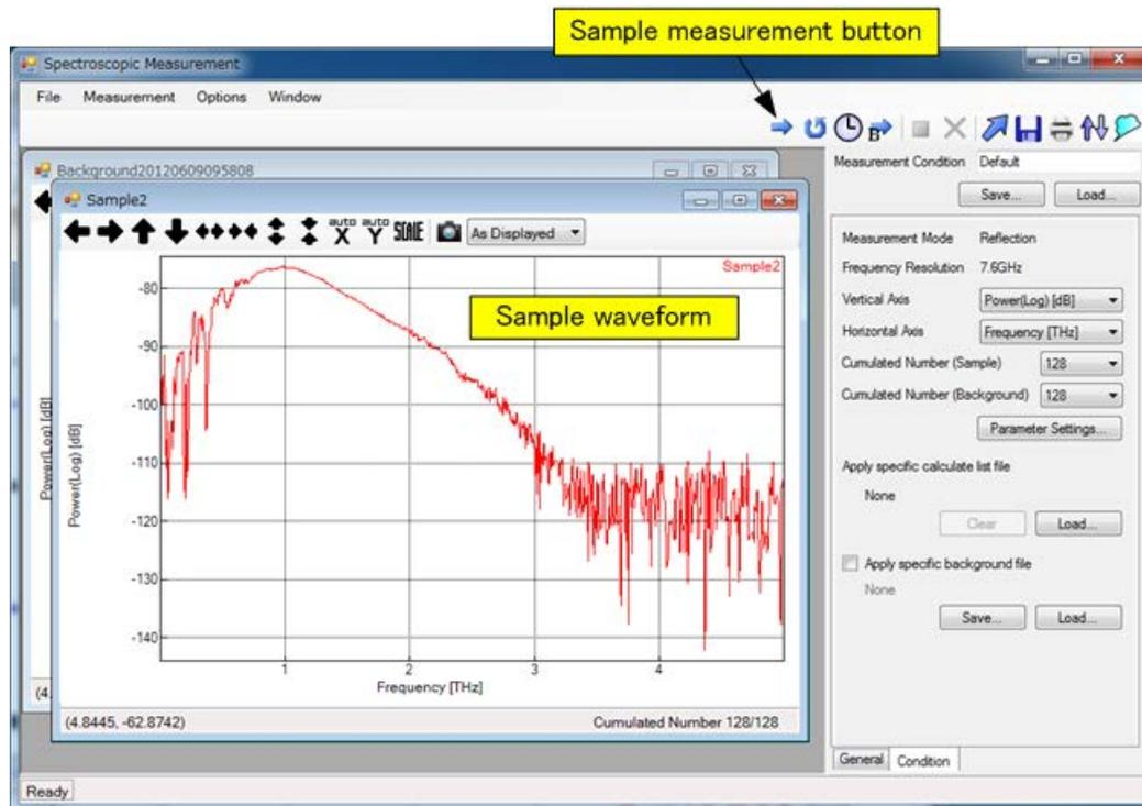
To continuously acquire and monitor the sample waveform, click the
