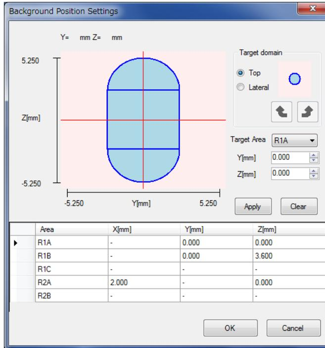
To use a reference for which multipoint background data settings are valid, insert the reference at the R1 position in the cassette to execute background measurement.
