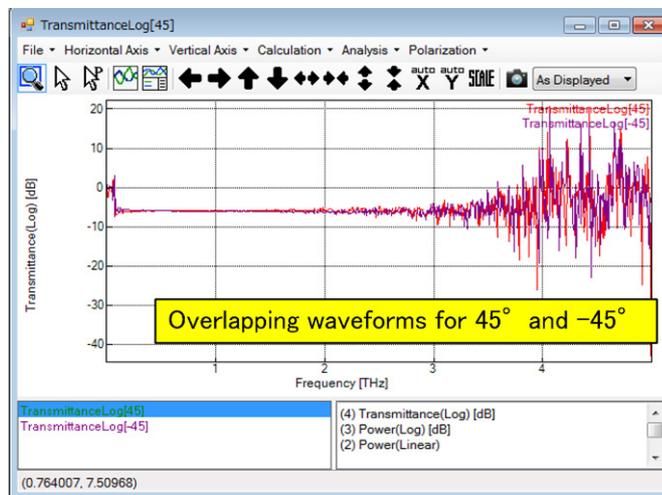
In the analysis window, the polarization analysis data can be displayed using various axes. The desired axes can be selected from the Polarization menu in the graph window.
