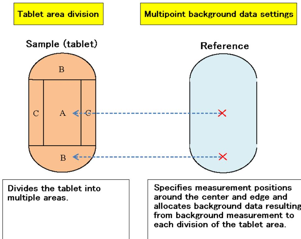
When applying background data acquired using multipoint background data settings to a tablet the area of which is divided for sample measurement, set On to Multiple Background Data Setting in 5. 2. 4. 2 "Condition Tab" on page 5-26.
