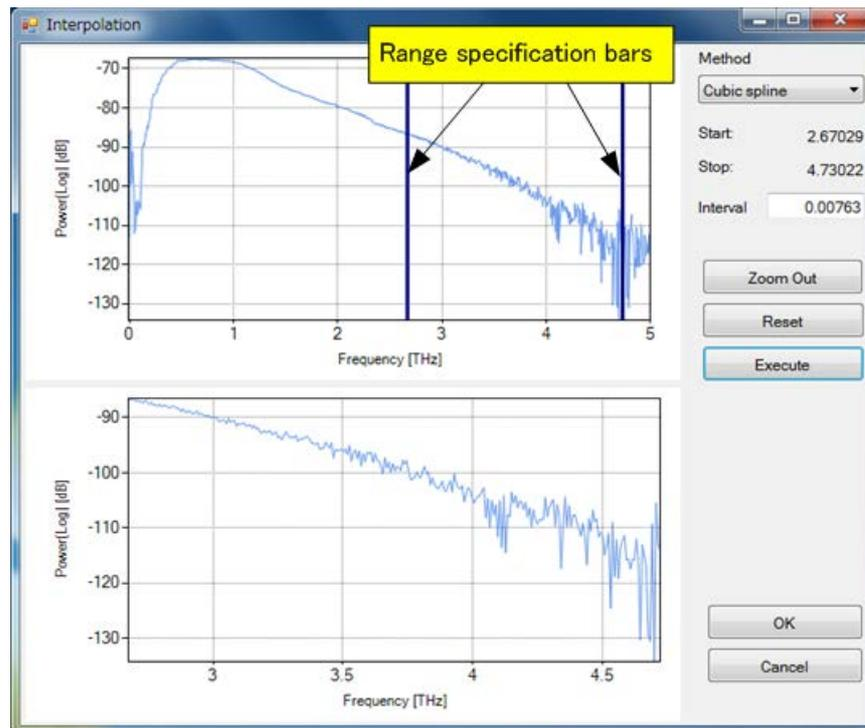
The graph on the top is the one before calculation. The graph on the bottom is the one after calculation.
