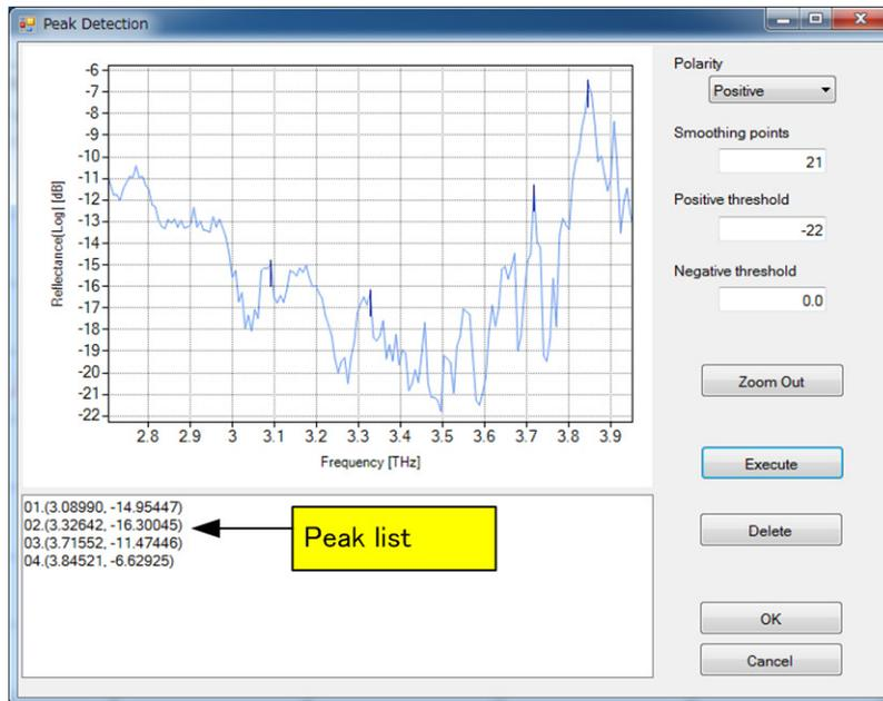
Clicking the **[OK]** button at this point displays labels (horizontal axis values) at the positions of the relevant peaks in the graph window.
