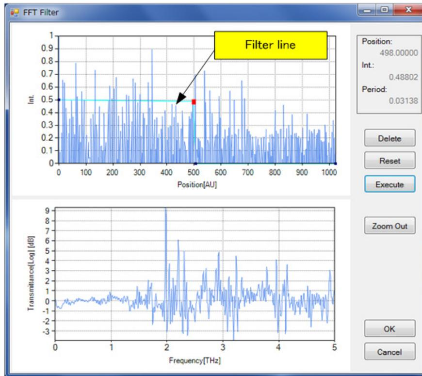
The graph on the top is the one after FFT. The graph on the bottom is the one after calculation.
