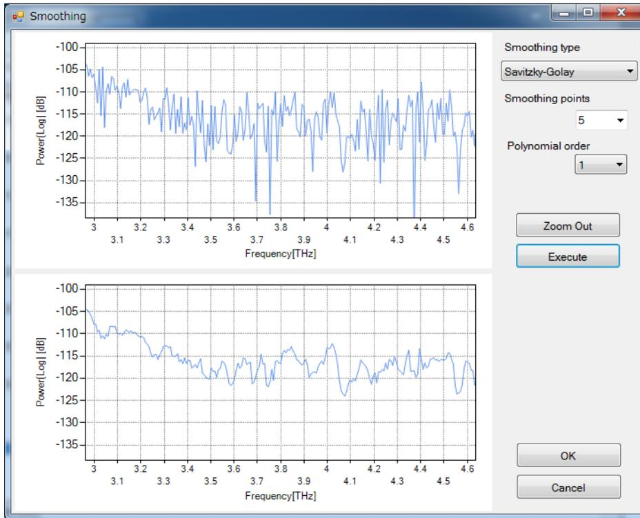
The graph on the top is the one before calculation. The graph on the bottom is the one after calculation.
