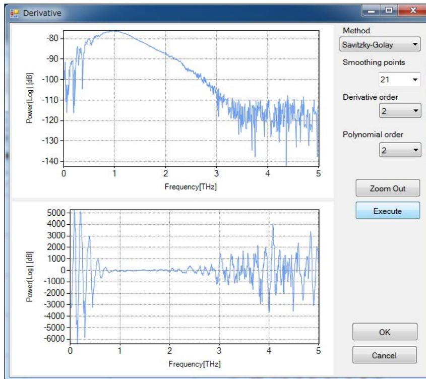
The graph on the top is the one before calculation. The graph on the bottom is the one after calculation.
