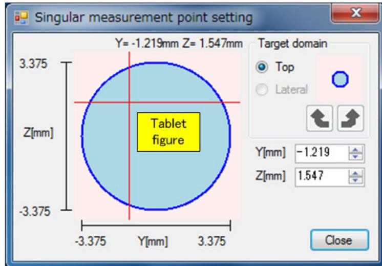
By clicking on the tablet figure, a point to be measured can be specified.
