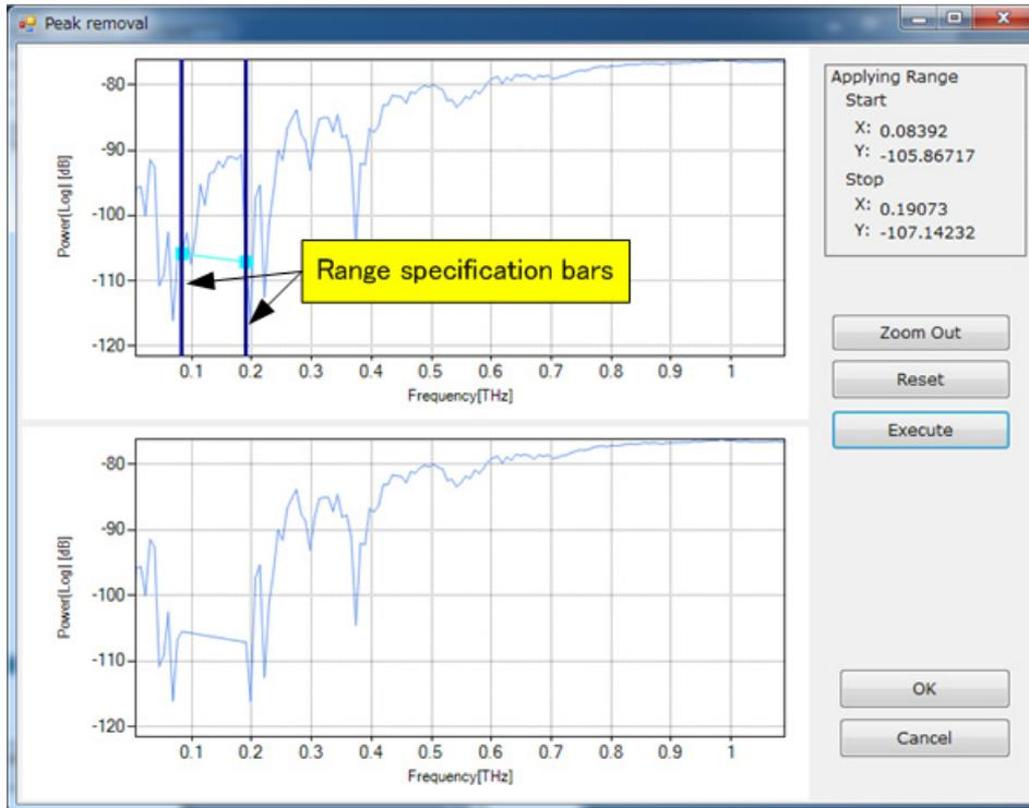
The graph on the top is the one before calculation. The graph on the bottom is the one after calculation.
