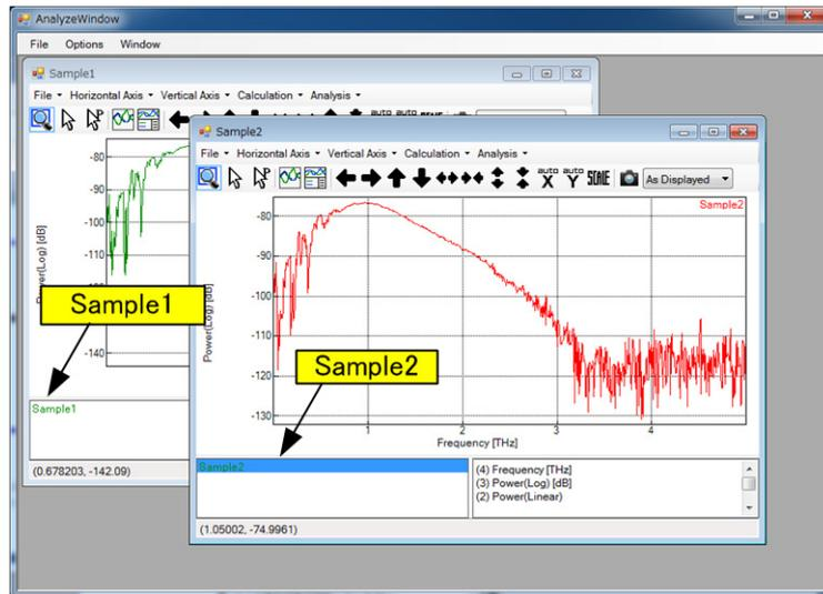
Select Sample2 with the mouse and press the [Ctrl and C] keys. Display the Sample1 window in front and press the [Ctrl and V] keys. The spectra in Sample1 and Sample2 then overlap.
