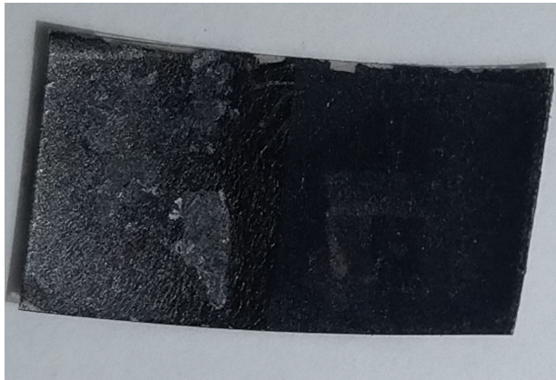
FIGURE 11. GO-rGO sample where some areas of the GO face on the left half of the sample were in contact with copper under short circuit, while other areas do not contact the metal. We compare the carbonyl absorption of these two areas.
